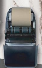
Molded of styrene and high impact polystyrene resin. One piece door construction. One piece back construction. Door is mounted to back with pivot posts and secured with replaceable locking fingers.
